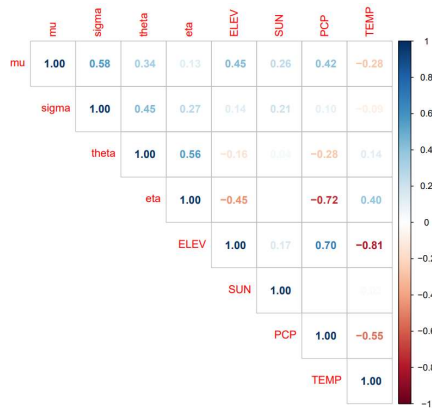
Figure A1 Cross-correlation between the selected local parameters (Koutsoyiannis and GEV parameters) for regionalisation and useful site characteristics that might act as an external drift information. Mu is the location parameter, sigma the scale parameter, theta and eta the Koutsoyiannis parameters, ELEV is short for elevation information, SUN is short for long term average of annual sunshine duration, PCP is short for long term average of annual rainfall amount, and TEMP is short for the long-term average of annual mean temperature.
