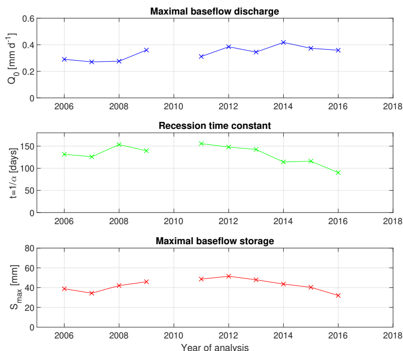
Figure 5. Temporal evolution of recession characteristics obtained from annual recession analysis, showing the results of the best fitted parameters for maximum baseflow ( Q_0 ), recession constant ( 1/\alpha ) as well as the first-order estimation of maximum baseflow storage ( S_{max} ).
