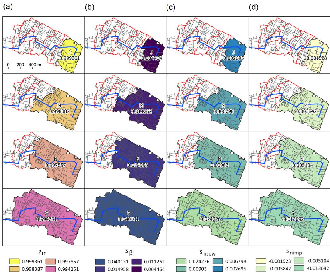
Figure 5. (a) Probability of specific flood volume ( $p_m$ ); (b) sensitivity coefficient  $S_\beta$ ; (c) sensitivity coefficient  $S_{nsew}$ ; (d) sensitivity coefficient  $S_{nimp}$  in sub-catchments J, M, N, S.
