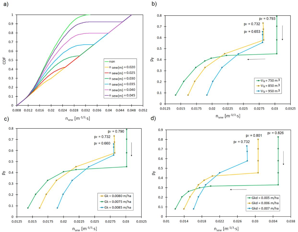
**Figure 9. (a) Empirical distributions of threshold values of Manning roughness coefficients of channels ( $n_{sew}$ ) for  $V_k = 950m^3$ . Impact of Manning roughness coefficient for channel on failure probability ( $p_F$ ) in relation to: (b)  $V_k$ , (c)  $G_d$ , (d)  $G_{kd}$ .**
