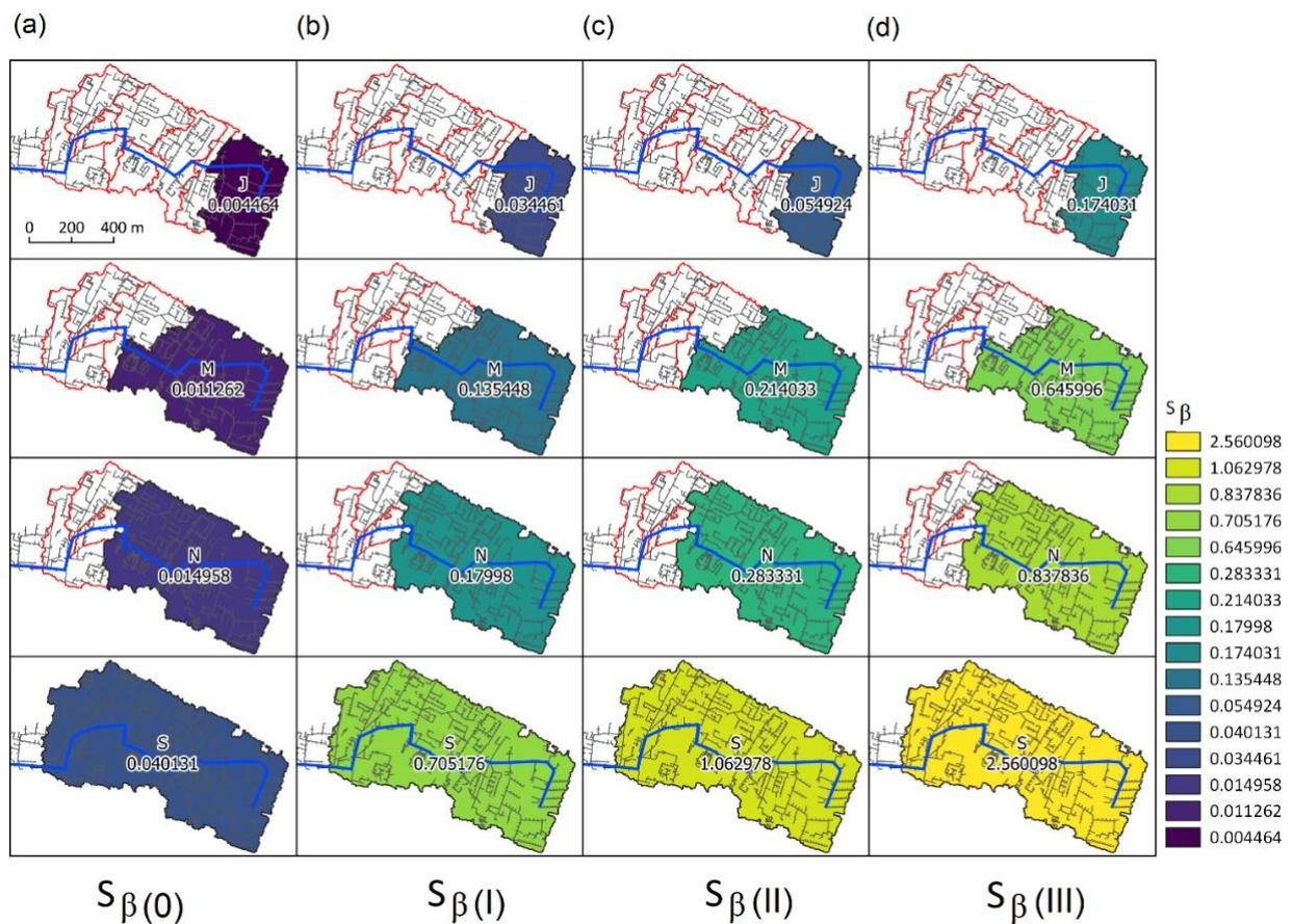
Figure 7. Sensitivity coefficient ( $S_{\beta}$ ) in sub-catchments for: (a) present state (0) and for (b) I, (c) II, (d) III corrective variants.
