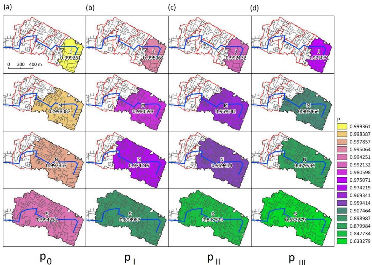
Figure 6. Probability of specific flood volume in sub-catchments for: (a) present state ( $p_0$ ) and for (b) I, (c) II, (d) III corrective variants.
