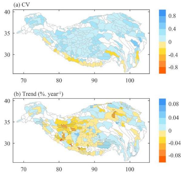
**Figure R6** Spatial distribution of (a) the Coefficients of Variation (CVs) and (b) trends for annual RPGs during the period from 1980 to 2018. CVs and trends at sub-basins with missing RPGs during the analysis period were filled with white color. The dots represent trends significant at the 95% confidence level.
