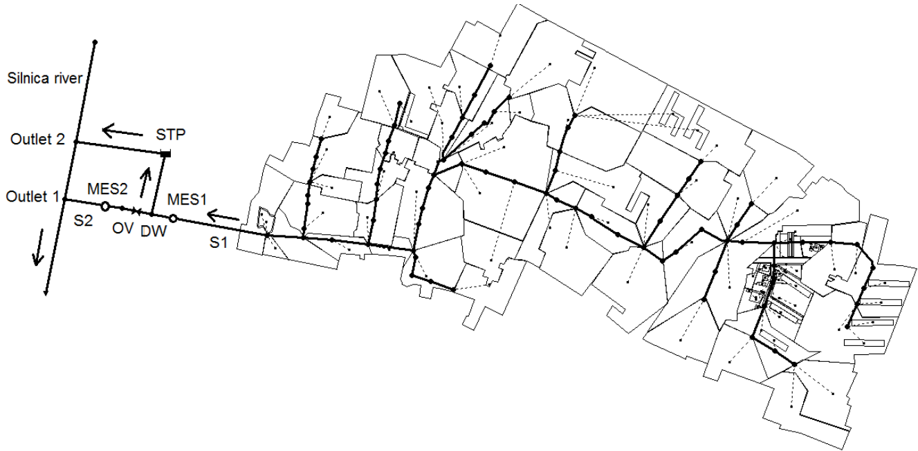
175 Figure 1. Scheme of the hydrodynamic model of the catchment generated in the SWMM program.
