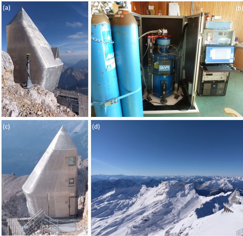
Figure 2: (a) The Zugspitze Geodynamic Observatory Germany (ZUGOG) with GNSS station in front; (b) OSG 052 installed on the ground floor at ZUGOG, (c) ZUGOG with snow height sensors and snow scale in front; (d) ZUGOG with a winter view of a part of the alpine research catchment Zugspitze including the Northern and Southern Schneeferner glaciers.
