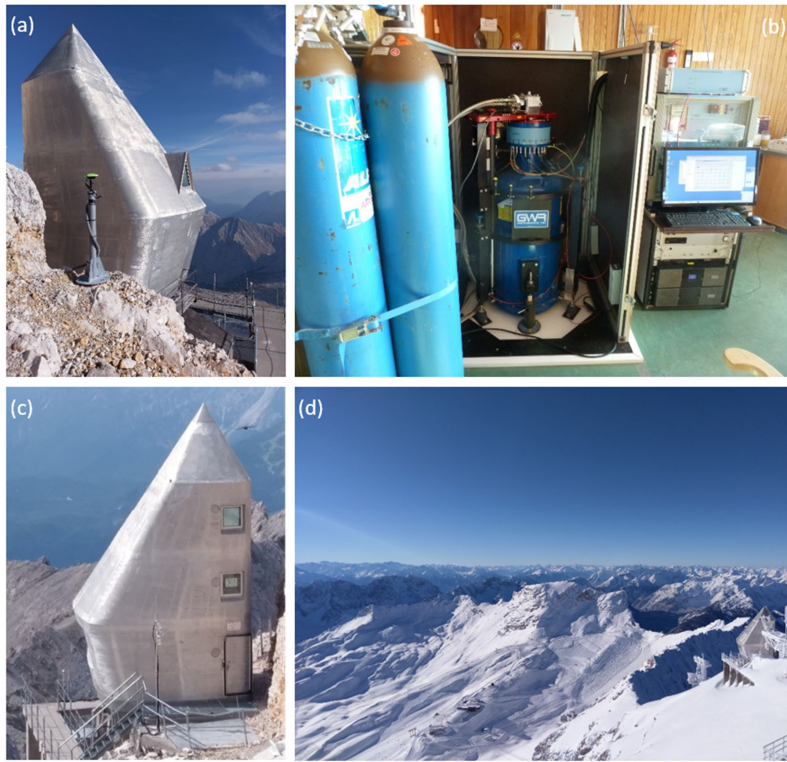
315 Figure 2: (a) The Zugspitze Geodynamic Observatory Germany (ZUGOG) with GNSS station in front; (b) OSG 052 installed on the ground floor at ZUGOG; (c) ZUGOG with snow height sensors and snow scale in front; (d) ZUGOG with a winter view of a part of the alpine research catchment Zugspitze including the Northern and Southern Schneeferner glaciers.
