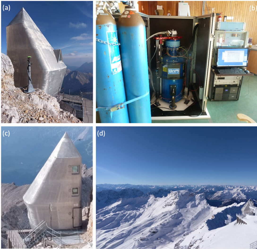
Figure 2: Top left: (a) The Zugspitze Geodynamic Observatory Germany (ZUGOG) with GNSS station in front; top right: (b) OSG 052 installed on the ground floor at ZUGOG, bottom left: (c) ZUGOG with snow height sensors and snow scale in front; bottom right: (d) ZUGOG with a winter view of a part of the alpine research catchment Zugspitze including the Northern and Southern Schneeferner glaciers.
