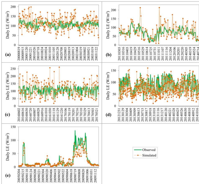
Figure 5: Observed and simulated daily LE series by the sine function upscaling method at tropical regions. Note: a to c represent BR-Sa3, GH-Ank, ID-Pag, located at the tropical rainforest climate region; d and e are the sites of PH-RiF and SD-Dem, located in the tropical monsoon and grassland climate regions, respectively.
