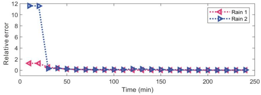
Figure 2: Relative error of flood predictions at different time steps.
