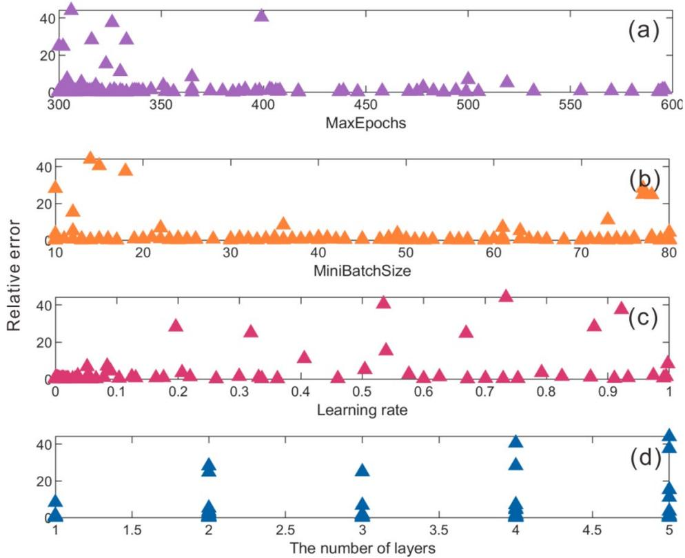
Figure 8: Influence of four types of network parameters on model prediction performance (i.e., relative error).
