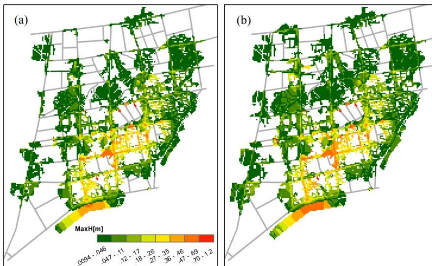
Figure 6: Sample comparison of flood maps of (a) ground truth and (b) model prediction in the new case study under a 50-yr event.
