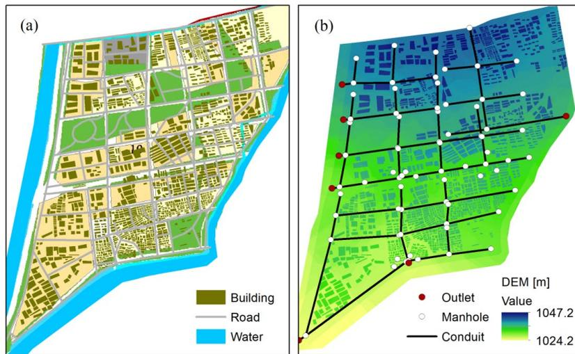
Figure 5: (a) landuse and (b) drainage network and DEM of the new case study.
