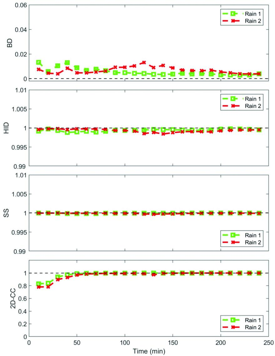
Figure 3: Degree of similarity (BD, HID, SS and 2D-CC) of the flood predictions of testing rainfalls at different time steps. Specifically, the closer the BD is to 0, and the HID, SS, 2D-CC are to 1, the better the prediction performance.
