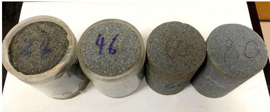
197 Figure 2. Physical drawing of permeable stones with four different particle sizes.
