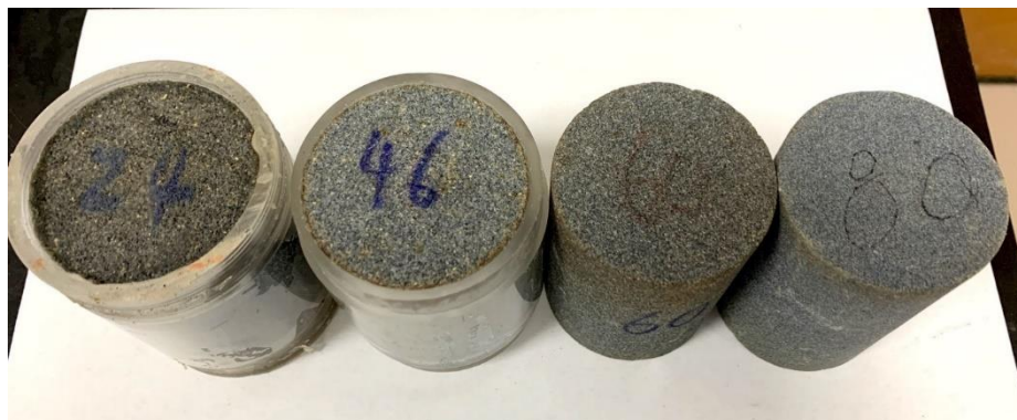
196 Fig. 2 Physical drawing of permeable stones with four different particle sizes.
