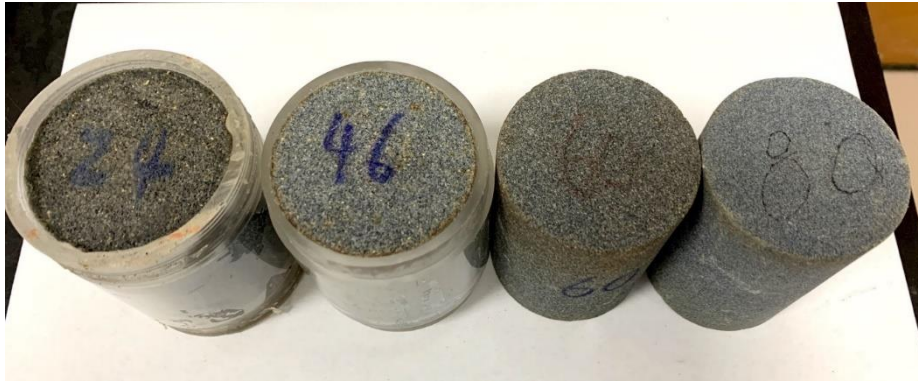
214 Figure 2. Physical drawing of permeable stones with four different particle sizes.
