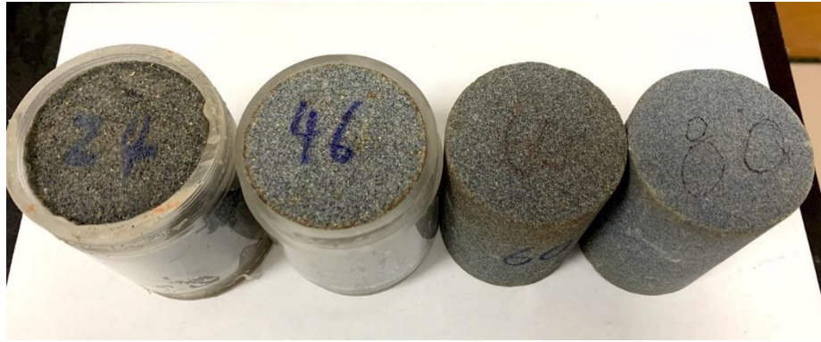
Fig. 2 Physical drawing of permeable stones with four different particle sizes.
