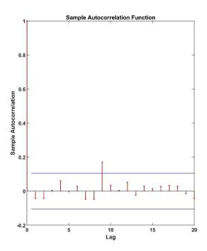
The PDS graph shows that except for two higher discharges, the peaks extracted at a threshold (T) of  $300 \text{ m}^3$ /s do not have any particular pattern, i.e., they tend to fluctuate randomly. The presence of these two higher values at 9 step time lag might be the reason for a higher correlation. But since most of the spikes are not statistically significant, this implies that the peaks are mainly independent of each other.
