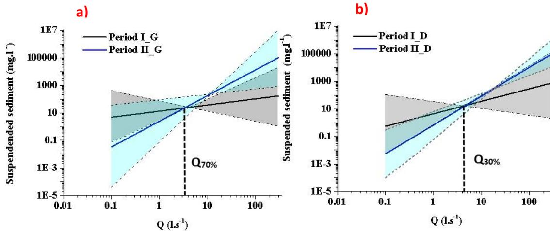
**Figure 7 Theoretical sediment rating curves (tSRC) for the growing seasons (a) and the dormant seasons (b) of Period I and II. Solid lines denote the 50 percentile of the tSRC for each period (i.e. tSRC<sub>50%</sub>). The grey area denotes the range of the predicted tSRC composed of 5 and 95 percentiles (i.e. tSRC<sub>5%</sub> and tSRC<sub>95%</sub>). Q<sub>30%</sub> and Q<sub>70%</sub> represent the flow conditions of 3.9 l.s<sup>-1</sup> and 2.0 l.s<sup>-1</sup>, respectively.**
