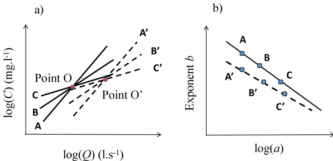
290 **Figure 2 Schematic showing a) how sediment rating curves (SRC) may rotate**
