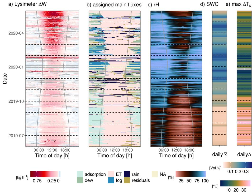
**Figure 2.** Diel and seasonal dynamics of a) lysimeter weight changes, b) assigned flux types, both from lysimeter 6, c)  $rH$  measured at 1 m height. Solid vertical lines mark sunrise and sunset, respectively, determined with the geographic coordinates of the field site. Mean  $SWC$  at 0.05 m depth and maximum diel difference of  $T_s$  are displayed as diel measurements in panels d) and e).
