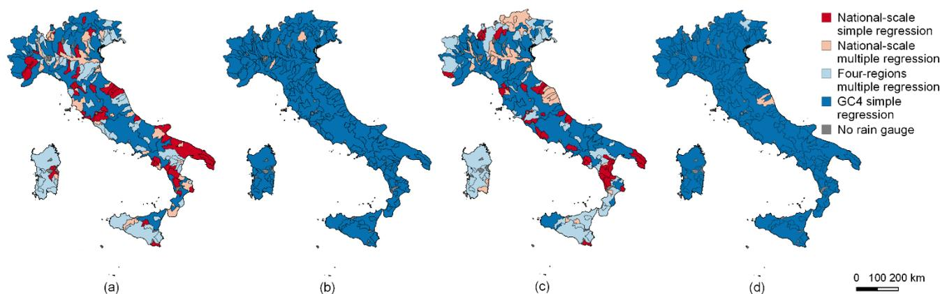
445 **Figure 6. Absolute bias assessment for all the regression models used for the 1-hour case (a,b) and 24-hour case (c,d). The color refers to the model that provides the lowest absolute value of the bias. The GC4 model bias in cases (a) and (c) was only evaluated for statistically significant areas, while it was evaluated over every area in (b) and (d).**
