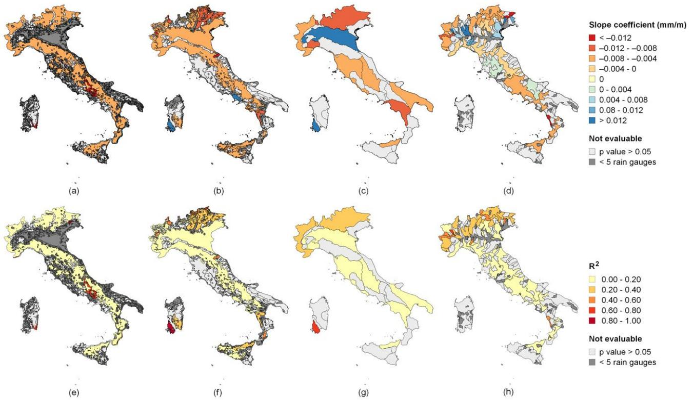
355 **Figure 4.** Slope coefficients of the regression between the mean 1-hour rainfall depth and elevation for GC1 (a), GC2 (b), GC3 (c) and GC4 (d); the  $R^2$  of the regression between the mean 1-hour rainfall depth and elevation for GC1 (e), GC2 (f), GC3 (g) and GC4 (h).
