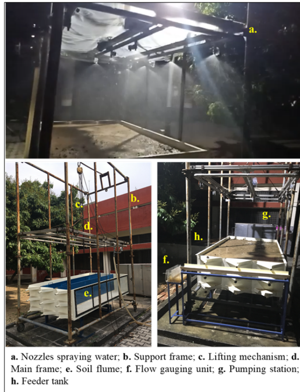
Figure 8. Designed rainfall simulator for moving storm experiments.
