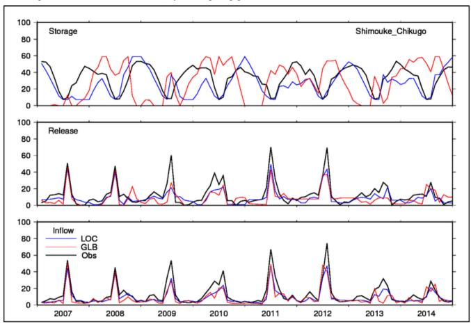
Figure 7 Reservoir operation at the Shimouke Dam on the Chikugo River. Top: monthly time series of water storage (10<sup>6</sup> m³ year¹). Middle: monthly time series of release (m³ year¹). Bottom: monthly time series of inflow (m³ year¹).
