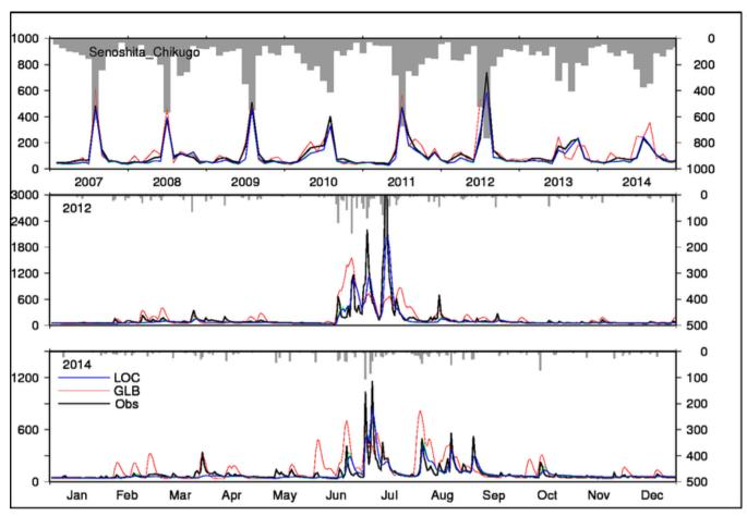
Figure 5 River discharge at Senoshita on the Chikugo River. Unit is m<sup>3</sup> s<sup>-1</sup>. Top: monthly time series of streamflow (lines) and basin-averaged precipitation in the LOC simulation (bars). Middle: daily time series of streamflow and precipitation in the wettest year of the validation period. Bottom: daily time series of streamflow and precipitation in the driest year of the validation period.
