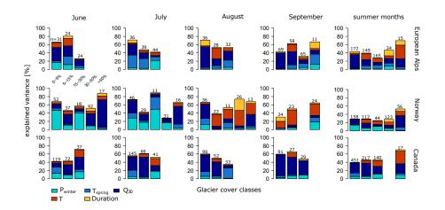
Figure 8. Explained variance of C during WD events for groups of catchments with similar glacier cover. No bar is present if there were less than 10 events for a gc class and month. The number above the bars indicate the number of events used in the regression model.
