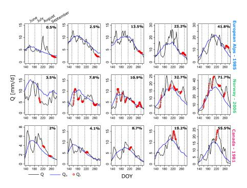
**Figure 3.** Examples of streamflow responses (Qr) to WD events in different catchments and in different months. Each row represents one region and one specific year. The columns are different catchments, they are sorted from low to high relative glacier cover (left to right). Note the different y-axis for some of the plots.
