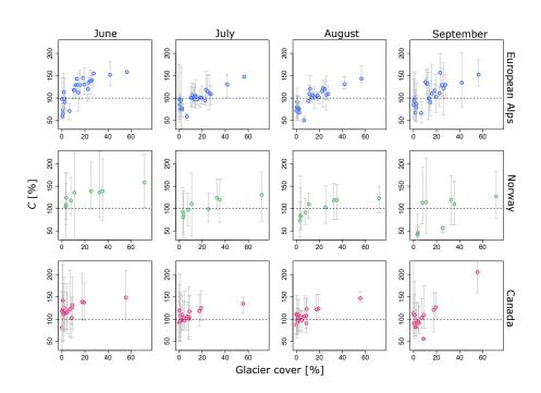
Figure 4. Level of compensation (C) during WD events for the different regions (rows) and the different months (columns) against gc of the different catchments. The coloured circles indicate the mean response and the gray bars show the range of C, i.e. the minimum and maximum C.
