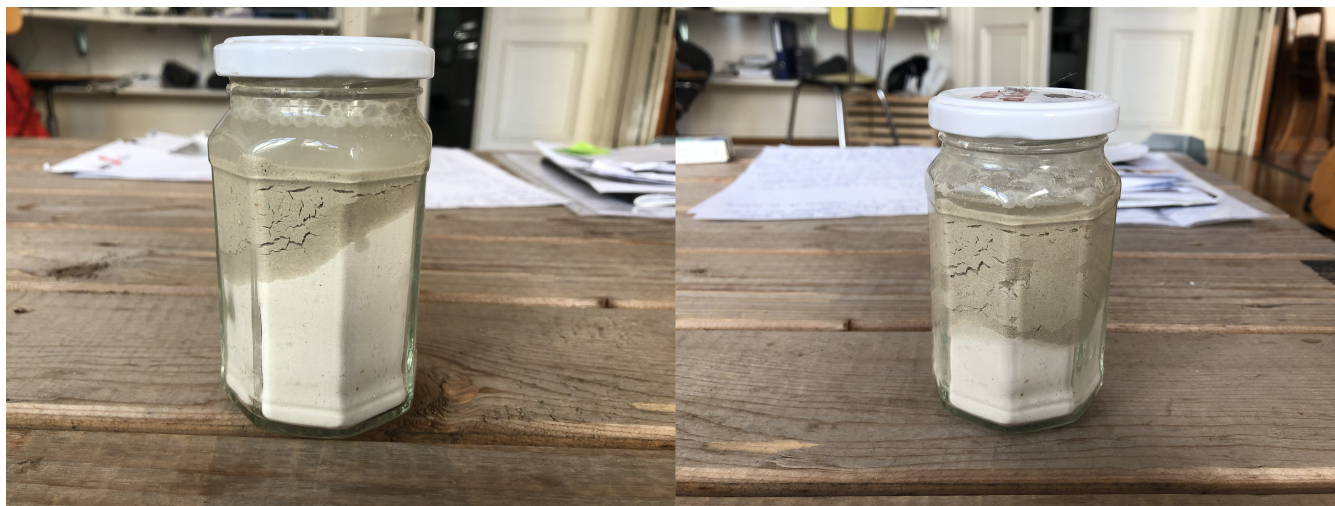
Figure 2. Do-it-yourself infiltration experiment with a sand column. Water is poured at the top of the column, and the panels show the infiltration after five minutes (left) and one hour (right). Note the sharp gradient in the transition from wet to dry sand - the so-called wetting front. The propagation velocity of the wetting front determines the infiltration rate and hence the amount of ponding water on the surface.
