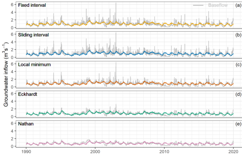
Figure 12. The comparison between the simulated groundwater inflow and the separated baseflow in the Zwarte Beek.
