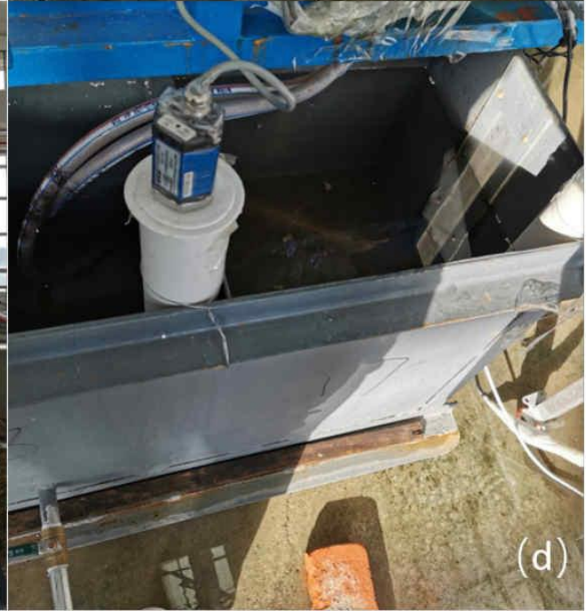
Figure 2: Laboratory apparatus. (a), (b), (c) and (d) show the overall experimental device, the electric fan system, the wind speed measuring device, and the flow measuring device, respectively.
