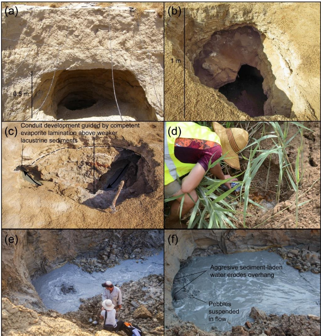
5 Figure 8: Field impressions of conduits and karstic groundwater springs at Ghor Al-Haditha. (a) Nested sinkhole in the alluvium (located in the southern part of the uvala) intersecting a further cavity or pipe. Photo: Damien Closson, 2008. (b) Sinkhole in lacustrine mudflats (located just inland of CM7; photo taken 2018) with pipe disappearing toward the top of the picture. (c) Conduit 10 formed in lacustrine mudflat deposits near to the shoreward termination of CM1 (photo taken 2014). The flow has excavated a conduit in the weaker mud deposits below a more competent evaporite lamination. (d) Spring s_4 at CM5 at base flow rate (estimated discharge: 2 \times 10^{-4} \text{ m}^3 \text{ s}^{-1} ). The main stream is fed by several similar seeps within the depression at the channel head. Photo taken: 2018. (e) s_4 during high flow three days after an intense rainfall event (estimated discharge: 2 \times 10^{-1} \text{ m}^3 \text{ s}^{-1} ). Photo taken: 2015, modified after Al-Halbouni et al. (2017). (f) Close-up of s_4 during high flow. The nature of the sediment load varies from fine sediments to pebble-sized clasts (up to 5 cm diameter). Photo taken: 2015, modified after Al-Halbouni et al. (2017).
