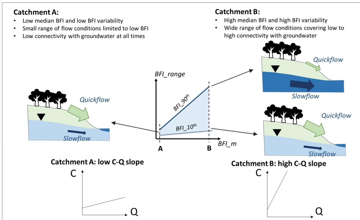
Figure 7. Conceptual diagram of the expected hydrological conditions in catchments with low and high median and variability in baseflow contribution ( $BFI_m$  and  $BFI\_range$ ), as Catchments A and B, respectively. The contrasting hydrological conditions can help explain our modelled results of the impacts of baseflow contributions on C-Q slopes. Note that the C-Q intercepts in the plots are not indicative since we do not investigate the variation in C-Q intercepts in this study.
