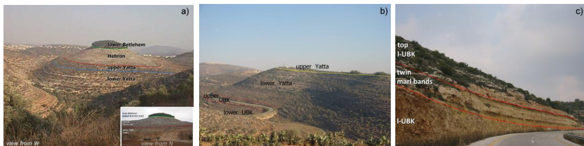
Figure 3. Correlation of landform and lithology. Nabi Ghayth hill, west of Beitillu (a); Nabi Aneer spring group (b). Twin marl band underlying a local perched aquifer (c).
