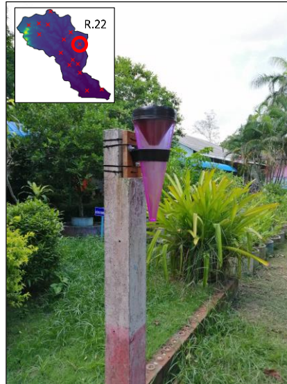
Figure A1: An example of installing a cone-shape transparent plastic citizen rain gauge at location R.22, Map Tong school.
