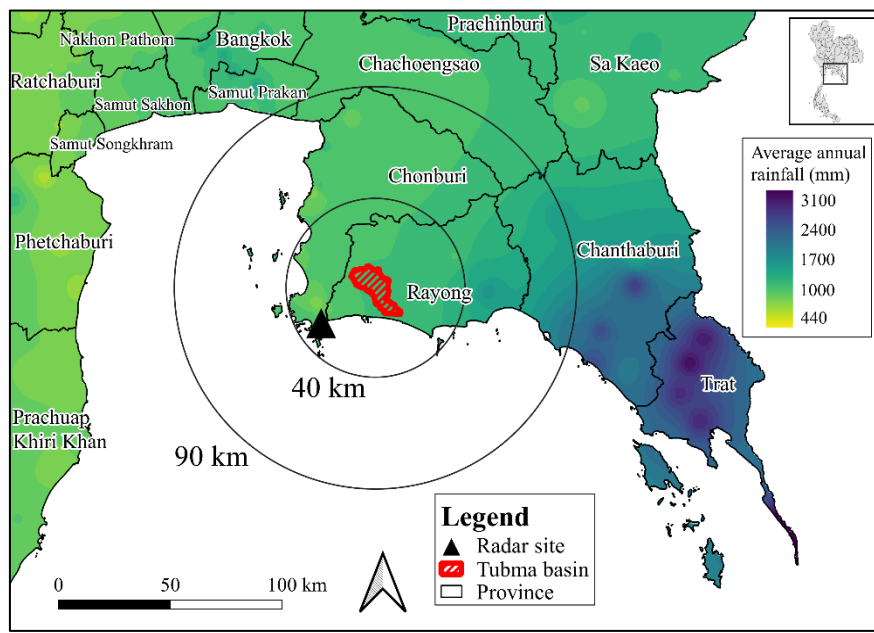
Figure 1: Climatological spatial rainfall distribution in and around the Tubma basin calculated from 30-year average annual rainfall data of 311 daily rain gauge network by using IDS method.
