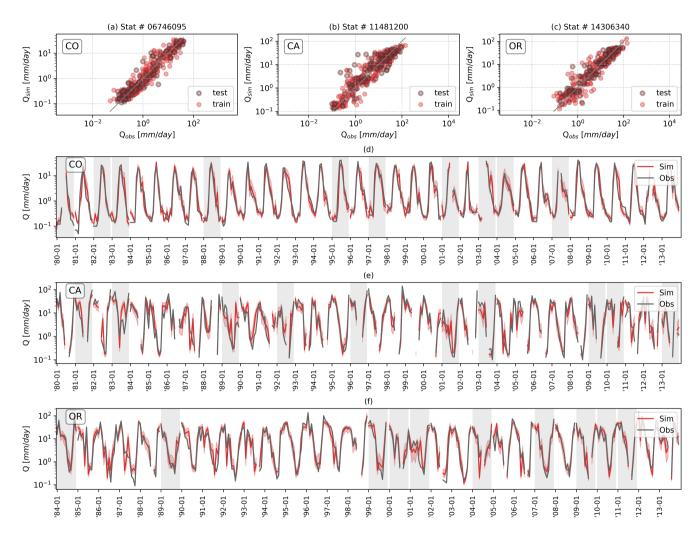
Figure 7. Comparison between monthly maximum river discharge simulations from run 1 and observations of three different catchments. The grey shaded areas indicate years belonging to the test-set. The shaded red areas represent the simulation confidence interval evaluated as the  $5^{th}$  and the  $95^{th}$  percentile.
