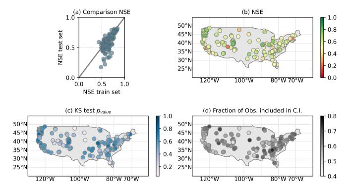
Figure 6. Performances of the SN-1 network in terms of NSE for the 159 catchments having NSE  $\geq$  0.5 in the testing process. Panel (a) compares the performances of the training- and test-set. Panel (b) shows the value of NSE per catchment. Panel (c) shows the  $p_{value}$  resulted from the KS-test per catchment. Panel (d) shows the overall fraction of observations falling inside the estimated discharge uncertainty bounds per catchment.
