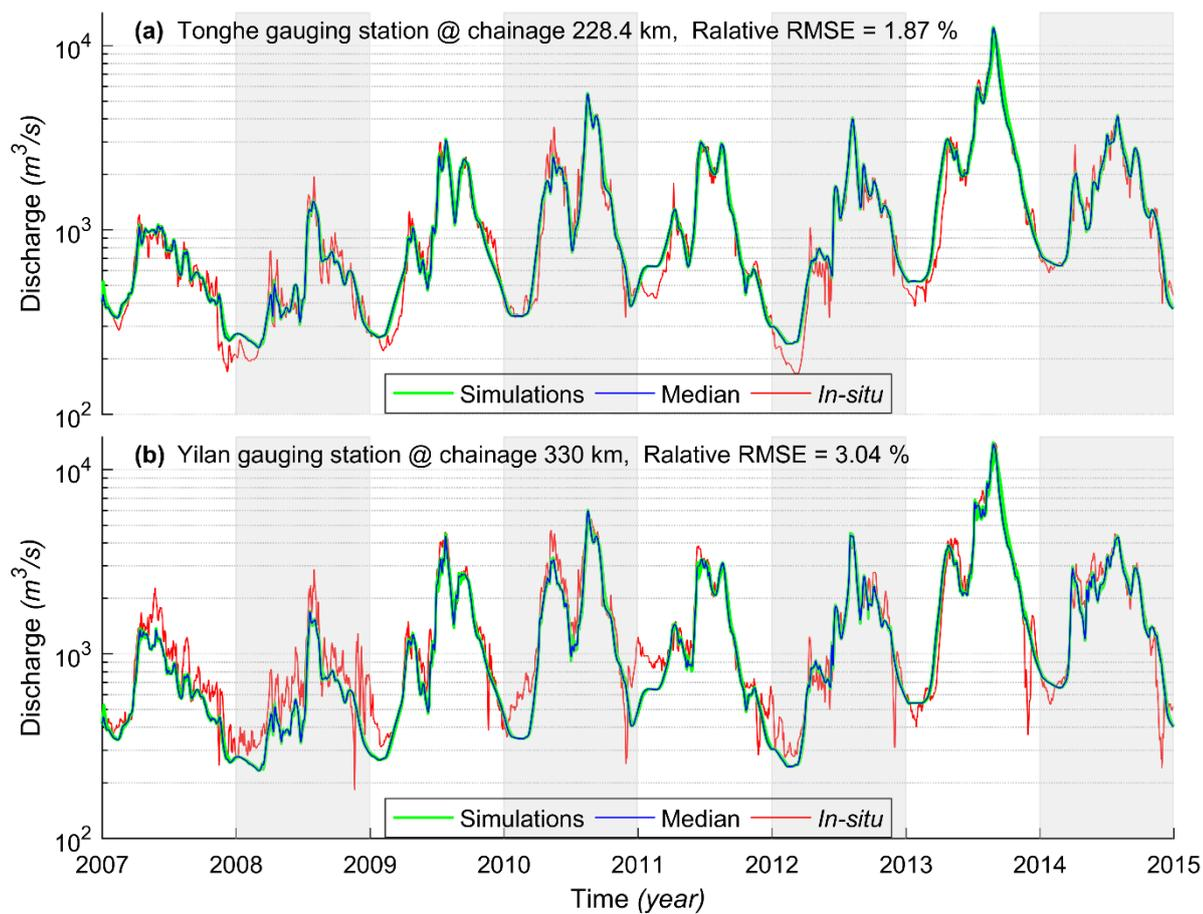
**Figure C1.** Validation of simulated discharge at two gauging stations. Note, in each plot, results of the median and individual simulations of an ensemble of 30 calibrations (i.e. calibration #1, #2, and #3) are shown.
