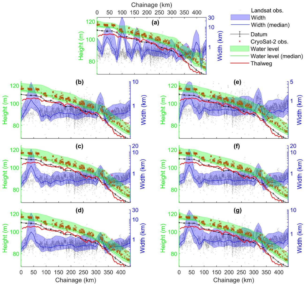
450 **Figure C2.** Comparison of model simulated water level, width, and datum using different calibration data sets. (a) calibration #1; (b) calibration #2a; (c) calibration #2b; (d) calibration #2; (e) calibration #3a; (f) calibration #3b and (g) calibration #3. Note, y axes are in log scale. Color bands indicate the boundary (i.e. maximum and minimum) of simulations. Along with model simulations, satellite observations of WSE and width are plotted.
