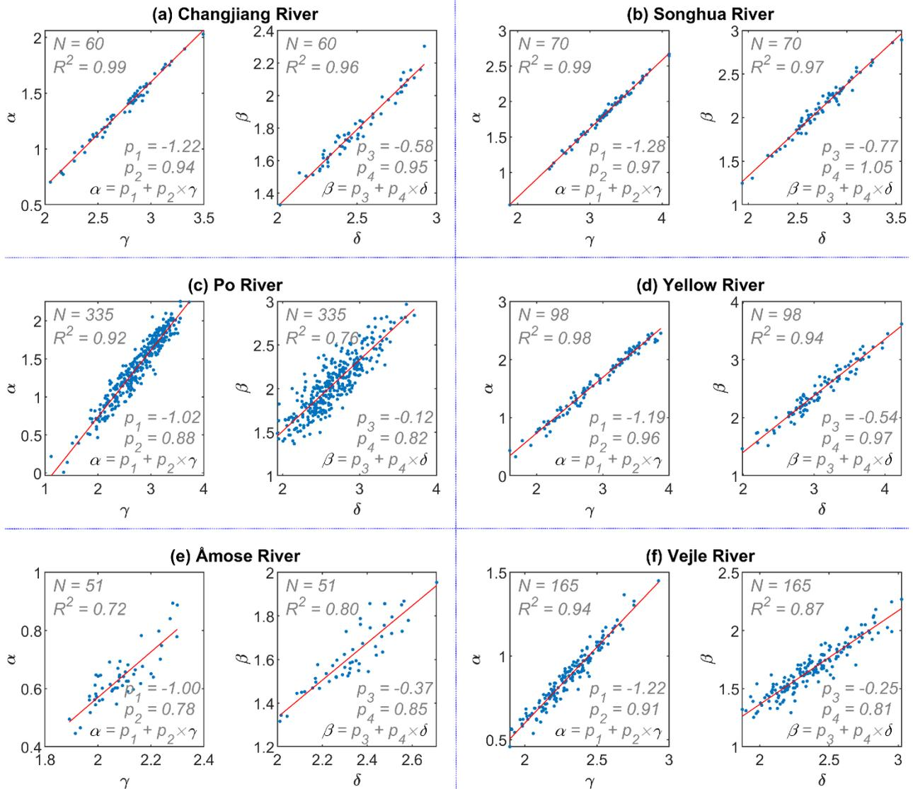
420 **Figure A4.** Linear relationships between gamma ~ alpha and delta ~ beta for six rivers. Randomly generated Manning's coefficient in range of 0.015 ~ 0.05 for each cross-section was used to calculate conveyance. The number of cross-sections, coefficient of determination, and regression coefficients are labelled in each plot.
