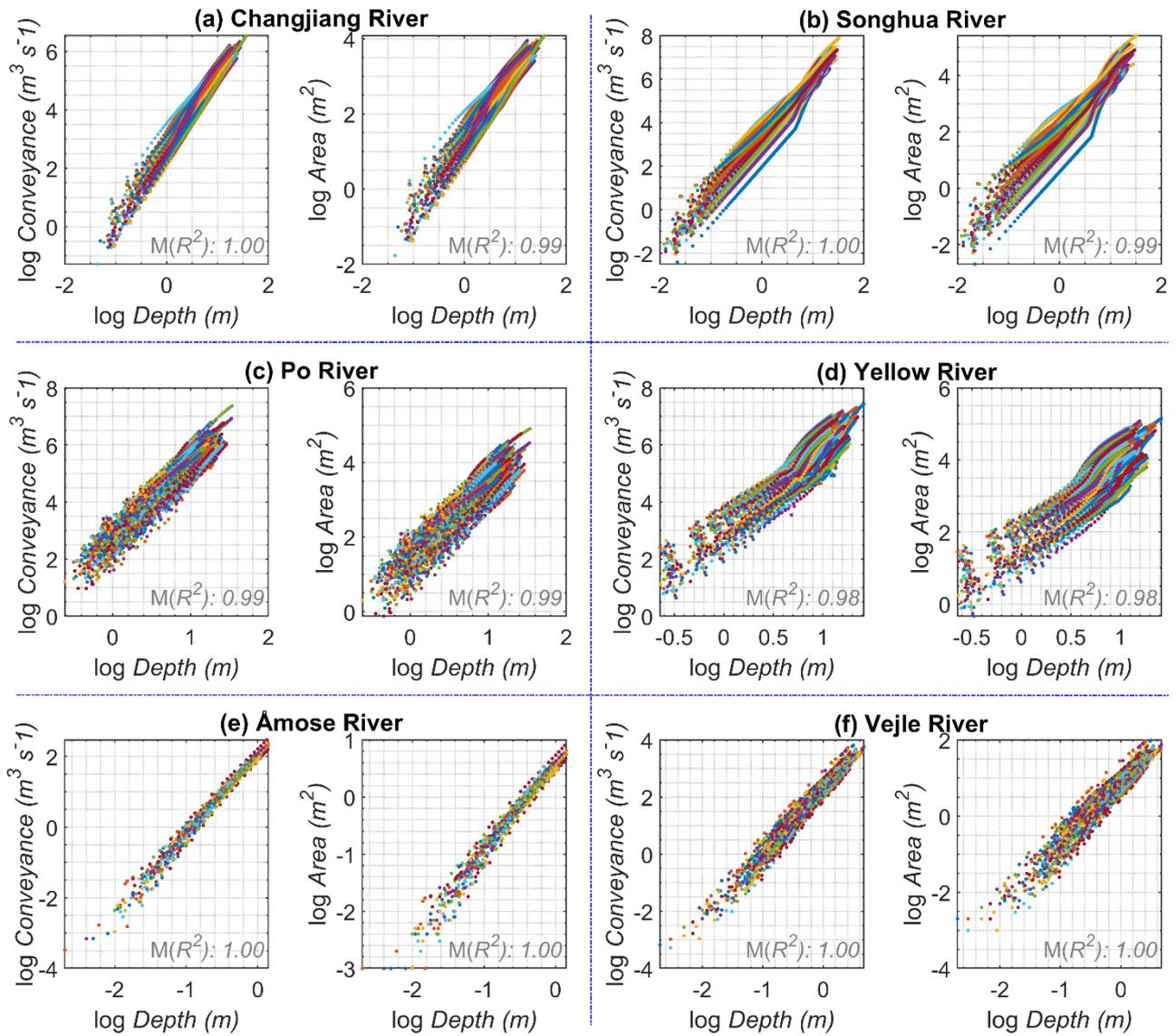
**Figure A2.** Relationship between logarithmic depth and logarithmic area and logarithmic conveyance. Similar to **Figure 1** but a uniform Manning's coefficient of 0.03 was used to calculate conveyance. This results in a stronger linear relationship. However, a uniform Manning's coefficient is not very realistic in natural rivers.
