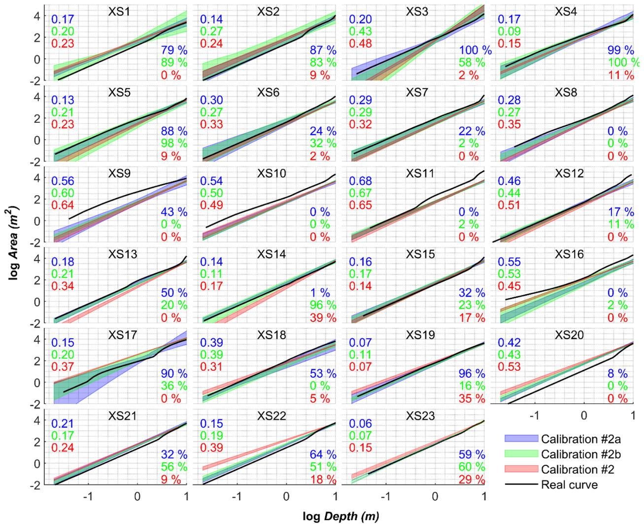
430 **Figure B2.** Calibrated curves using three scenarios of width observations only, i.e. one width observation per five-km reach
