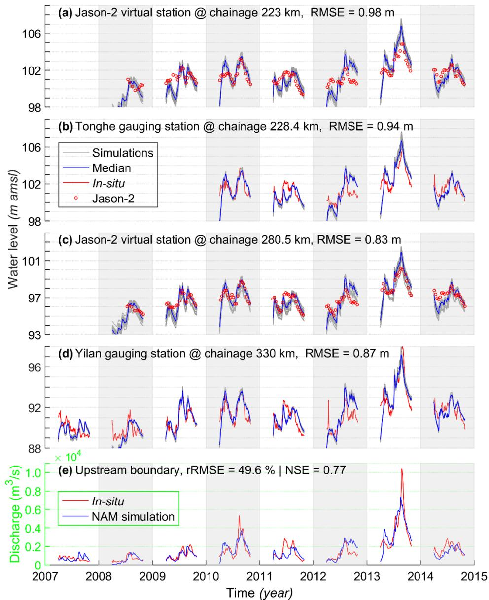
455 **Figure C3.** Similar to **Figure 6**, but upstream boundary is rainfall-runoff model simulation instead of in-situ discharge, which are shown in (e). Note that, NAM model was not calibrated at this location.
