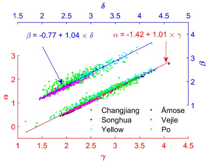
**Figure A3.** Linear relationships between gamma ~ alpha and delta ~ beta using data of all six rivers. Similar to **Figure 2**, but a uniform Manning's coefficient of 0.03 was used.
