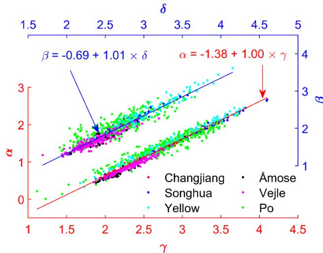
**Figure 2.** Linear relationship between  $\alpha/\beta$  and  $\gamma/\delta$ . Each dot represents one cross-section of a certain river. Dots of the same color are from the same river. Manning's coefficient for each cross-section is randomly generated between 0.015 and
