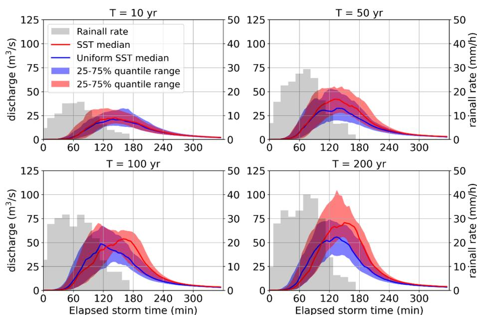
**Figure 5. Time series of simulated hydrographs for Franklinton based on the 3-h design storms from 10-yr to 200-yr return periods with spatially uniform (blue) and spatially distributed (red) rainfall. The grey bar indicates the median value of basin-averaged rainfall rate.**
