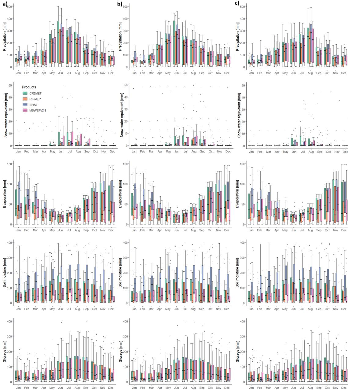
**Figure R17.** Mean monthly water balance components over rain-dominated catchments, obtained by forcing the TUW model with different  $P$  products for the: *a*) calibration (2000–2014); *b*) Verification 1 (1990–1999); and *c*) Verification 2 (2015–2018) periods. The mean monthly  $P$  was added for comparison purposes.
