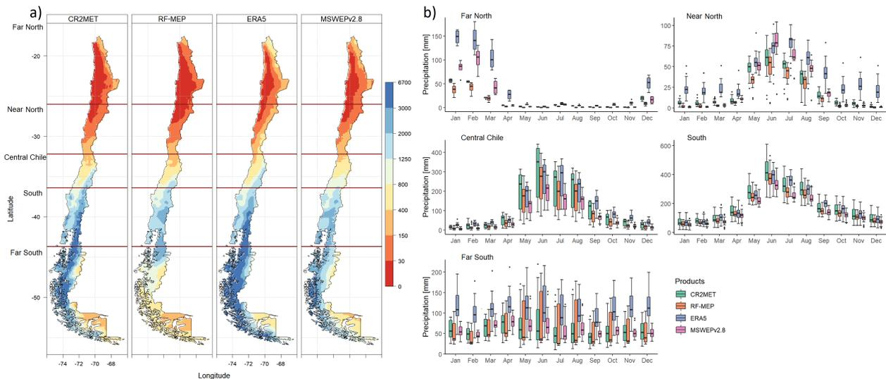
**Figure R2.** Comparison of  $P$  products over 2000–2014 (near-normal): *a*) mean annual  $P$  for each product resampled to a  $0.05^\circ$  spatial resolution using the nearest neighbour method. The dark red horizontal lines represent the limits of each major macroclimatic zone; and *b*) mean monthly  $P$  averaged over each catchment located within each macroclimatic zone (see Figure 1d).
