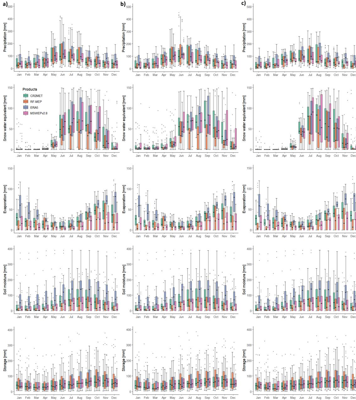
**Figure R15.** Mean monthly water balance components over nivo-pluvial catchments, obtained by forcing the TUW model with different  $P$  products for the: *a*) calibration (2000–2014); *b*) Verification 1 (1990–1999); and *c*) Verification 2 (2015–2018) periods. Mean monthly  $P$  was added for comparison purposes.
