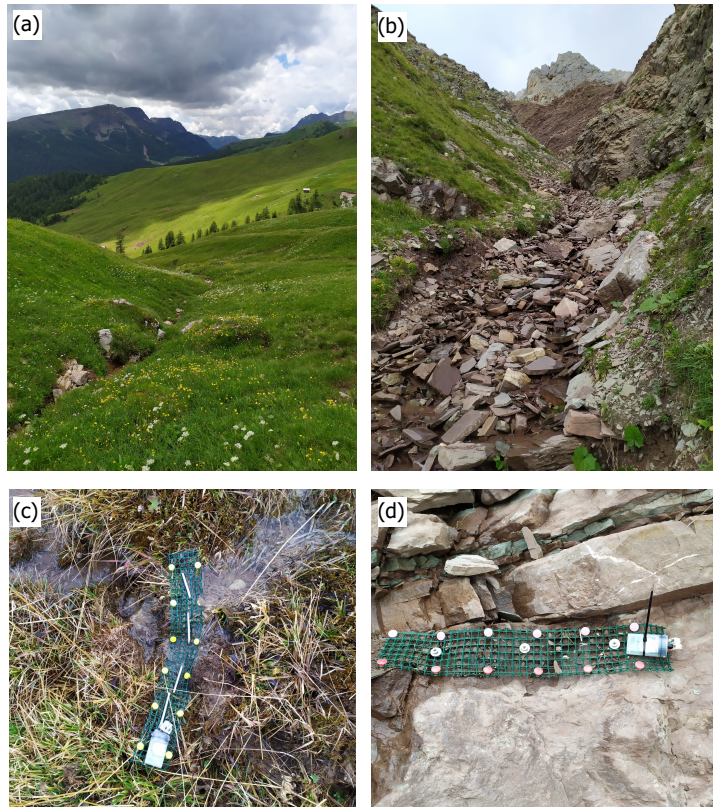
Figure 2. Left: picture of Zone 1 (a) and a sensor on the grass (c). Right: picture of Zone 2 (b) and a sensor' net screwed on a rock (d).
