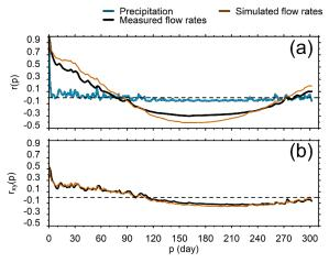
Figure 7: Autocorrelation functions of precipitation, measured flow rates, and simulated flow rates (a) and cross-correlation functions between precipitation (input) and measured or simulated flow rates (outputs) (b). Both were performed on 1/3 of the 2015-2018 period (m = n/3).
