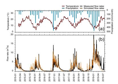
Figure 8: Measured meteorological data (a) and observed and simulated spring discharge (b).
