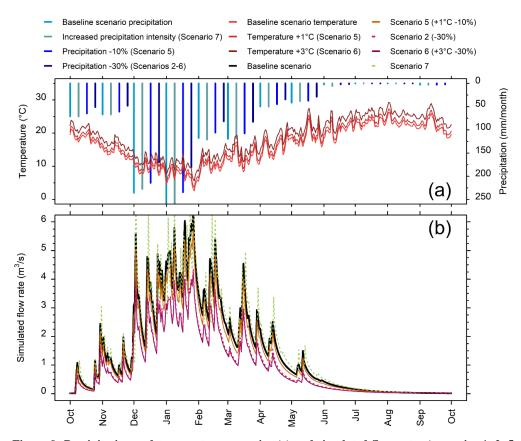
Figure 9: Precipitation and temperature scenarios (a) and simulated flow rates (scenarios 1, 2, 5, 6, 7, and the baseline scenario) for the spring for the 10th hydrological year of the period 2020-2030 (b).
