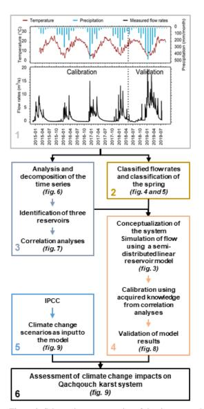
Figure 2: Schematic representation of the six-step methodology adopted for model conceptualization and the calibration.
