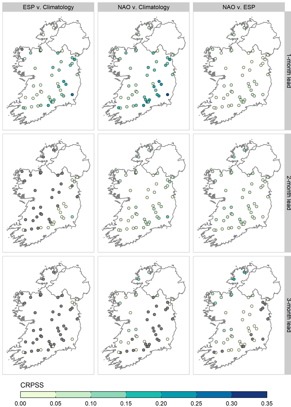
Figure 10. CRPSS values for historical ESP (left column), NAO-conditioned ESP (middle column), and the improvement made by NAO-conditioned ESP over historical ESP (right column), at lead times of 1, 2, and 3 months (rows). Catchments with negative skill (CRPSS < 0) are greyed out.
