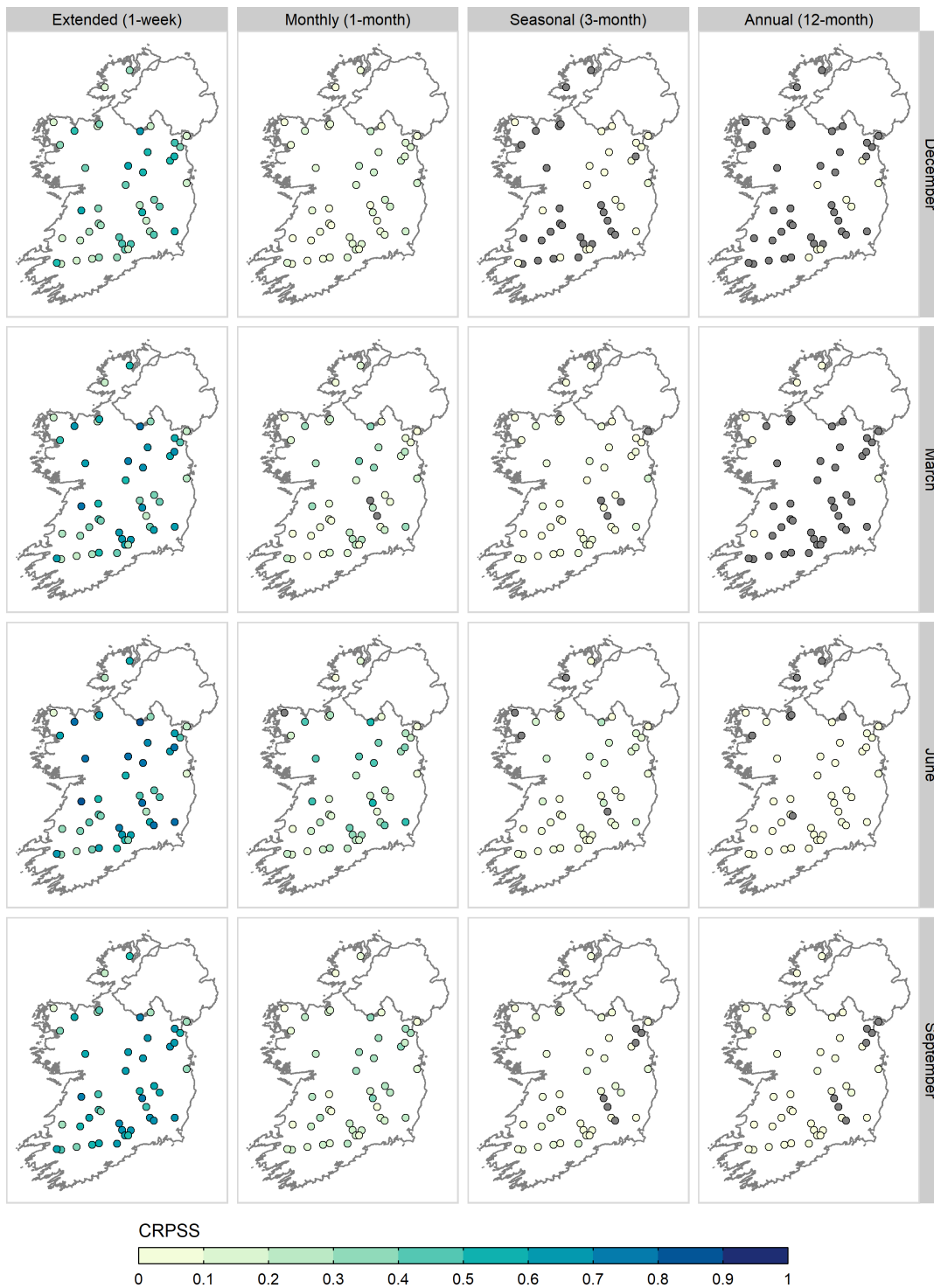
Figure 6. ESP skill for individual forecasts made at the 46 catchments for four sample lead times (columns) and four initialisation months (rows). Catchments with negative skill (CRPSS < 0) are greyed out.
