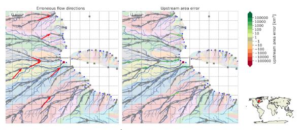
Figure C2: Largest exorheic basin (6830 km²) which is not resolved at 15 arcmin resolution indicated with highlighted basin outlet. See caption of Figure C1 for a full description.
