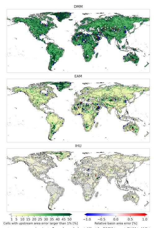
Figure 5: Relative upstream area error  $(\epsilon_{rel})$  at a 5 arcmin resolution (~10km) for DMM (upper), EAM (middle) and IHU (bottom). The background colors show the percentage of cells per 1x1 degree tile with a relative upstream area error of more than 1%, while the markers show the relative upstream area error at the outlets or sinks of the 500 largest basins globally (black lines).
