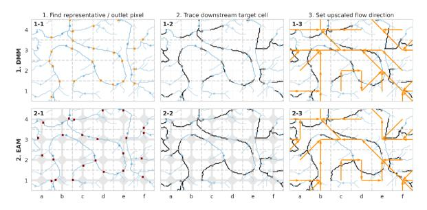
Figure A1: Visual explanation of the Double Maximum Method (DMM; first row) and Effective Area Method (EAM; second row). The target resolution grid (grey lines) and fine-resolution upstream area map (blue colors) are shown in all plots. The representative (EAM) or outlet (DMM) pixels (squares) are traced downstream until a criterium in a neighboring cell is met (black lines) and the upscaled flow direction are set (orange arrows).
