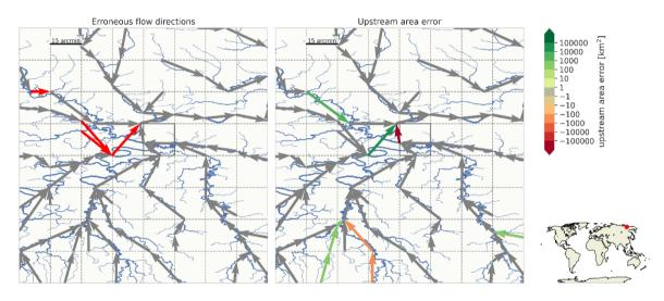
Figure C6: Second largest local upstream area error (-220876 km²) at 15 arcmin resolution indicated with highlighted cell. See caption of Figure C1 for a full description
