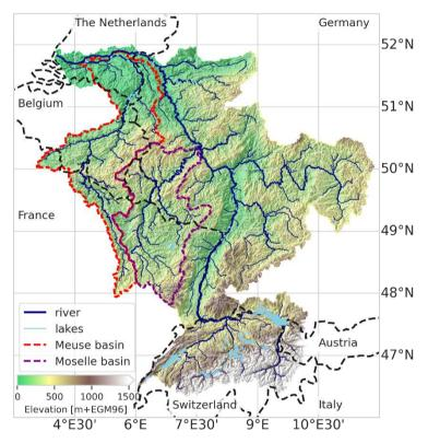
Figure 3: Study area: Rhine basin with average, elevation, rivers and basin outlines based on MERIT Hydro IHU 30 arcsec dataset (this paper); lakes are derived from the hydro Lakes dataset (Messager et al., 2016).
