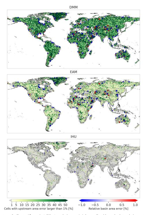
Figure D2: Percentage of cells at a 15 arcmin ( $\sim$ 30km) resolution per 1x1 degree tile with an absolute relative upstream area error of more than 1%, while the markers show the upstream area error at basin outlet and the black lines the outlines of the 200 largest basins globally.
