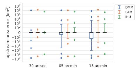
Figure 4: Absolute upstream area for DMM (blue), EAM (orange) and IHU (green) at three different resolution from 30 arcsec ( $\sim$ 1km; left column) to 15 arcmin ( $\sim$ 30 km; right column), where the black lines indicate the median error, the box the 25 -75 percentiles, the whiskers the 1-99 percentiles, the diamonds the 0.1-99.9 percentiles and the dots the min and max errors.
