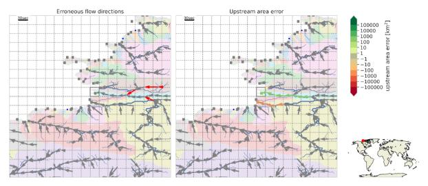
Figure C3: Largest basin (914 km²) with a relative upstream area error of more than 10% at 30 arcsec resolution indicated with highlighted cell. See caption of Figure C1 for a full description.
