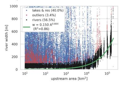
Figure B1: Fitted relationship between river width and upstream area for the river Rhine basin
