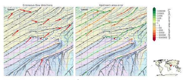
Figure C1: Largest endorheic basin (6996 km²) which is not resolved at 15 arcmin resolution indicated with highlighted basin pit.
