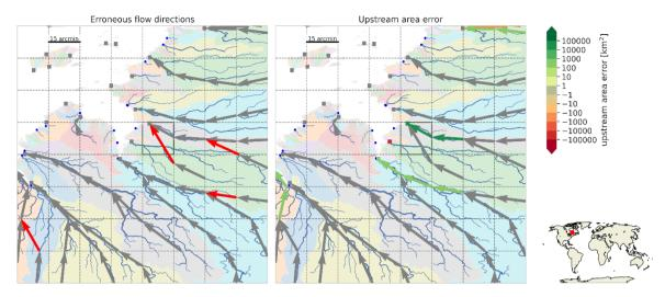
Figure C5: Largest basin (42017 km²) with a relative upstream area error of more than 10% at 15 arcmin resolution indicated with highlighted cell. See caption of Figure C1 for a full description.
