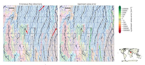
565 Figure C4: Largest basin (16717 km²) with a relative upstream area error of more than 10% at 5 arcmin resolution indicated with highlighted cell. See caption of Figure C1 for a full description.
