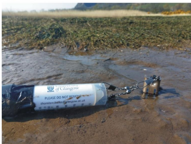
Fix logger to metal stake, protruding <1cm from tidal flat sediment
