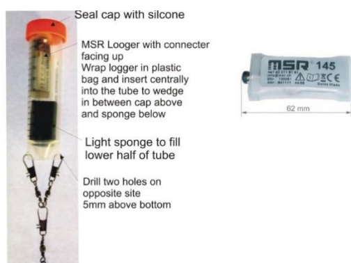
Figure A1: Mini Buoy components and installation
