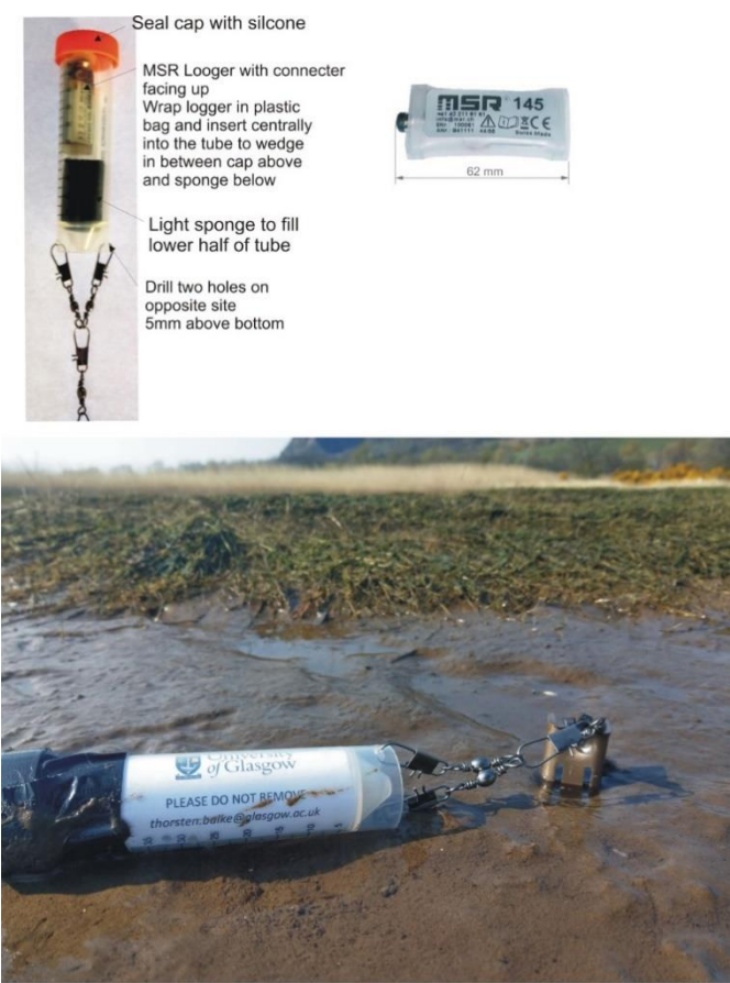
Figure A1: Mini Buoy components and installation
