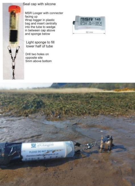
Fix logger to metal stake, protruding <1cm from tidal flat sediment
