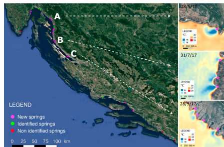
Figure 6. Springs reported in the literature (described SGD spring) vs new SGD spring identified with Landsat 8 TIRS. New SGD springs, not reported in the literature are represented with pink colour. Springs reported in the literature are represented with white colour.
