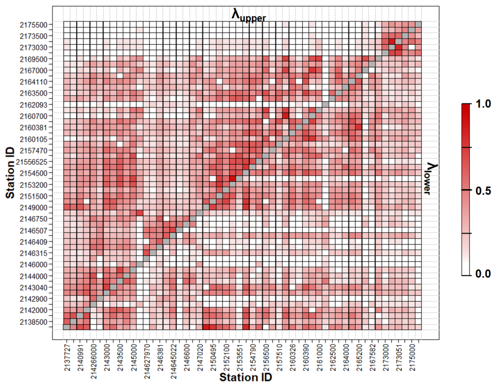
Figure 4 Pairwise upper and lower tail dependence for watersheds in the Yadkin-Pee Dee River Basin. The upper triangular matrix shows values for the upper-tail dependence and the lower triangular matrix presents values for the lower-tail dependence.
