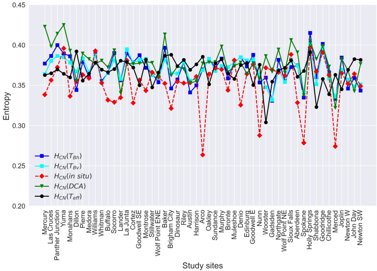
555 Figure 2 Entropies of in situ soil moisture, horizontally polarized brightness temperature ( T_{Bh} ), vertically polarized brightness temperature ( T_{Bv} ), soil effective temperature ( T_{eff} ) and DCA soil moisture across the study sites.
