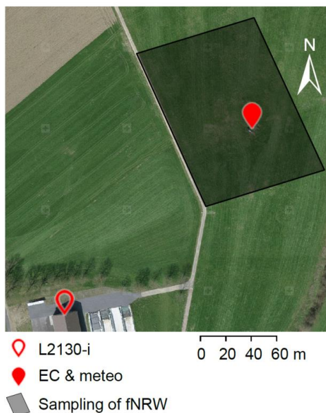
720 Figure A1. Measurements and sampling at the CH-CHA site (Satellite Image: © CNES /Spot Image/swisstopo, NPOC). “L2130-i” represents the isotopic compositions and mixing ratio measurements for ambient water vapor; “EC & meteo” represents the eddy-covariance and meteorological measurements; “Sampling of fNRW” represents the sampling of non-rainfall water droplets on foliage.
