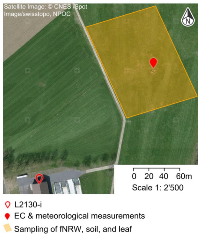
1115 Figure A1. Measurements and sampling at the Chamau site (Satellite Image: © CNES /Spot Image/swisstopo, NPOC). “L2130-i” represents the isotopic composition and mixing ratio measurements for ambient water vapor; EC, eddy covariance; fNRW, non-rainfall water on foliage.
