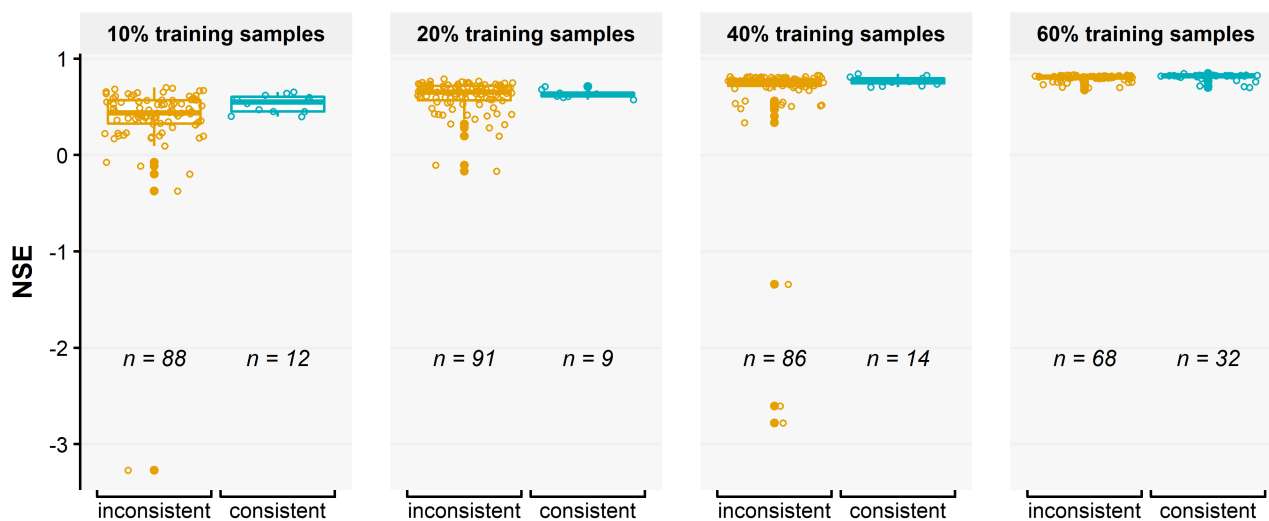
535 Figure 9 Boxplot of the prediction accuracy, as measured by Nash-Sutcliffe coefficient of efficiency (NSE), of the Washington Street SuDS site (WS) XGBoost models when samples of different sizes are used in model training. For each sample size, the models that offer consistent or inconsistent explanations are grouped together, and the numbers of consistent and inconsistent models (the n values) are shown. Observational SHAP values were used in the computation.
