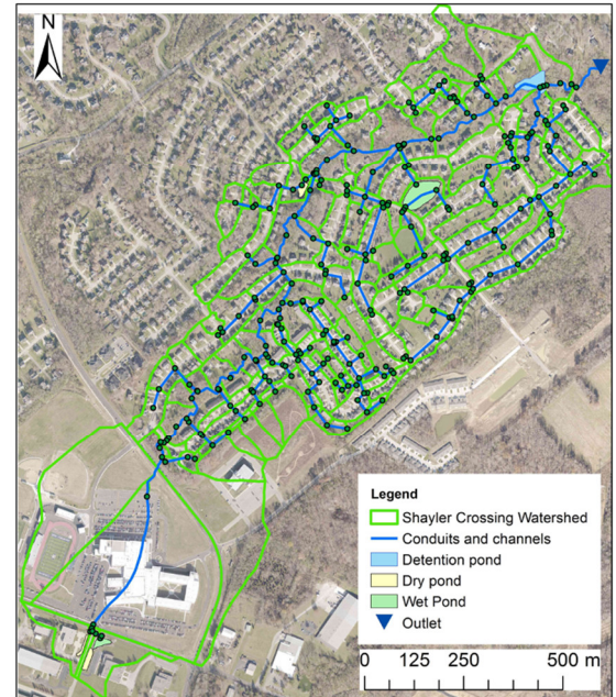
Figure 4 (a) Layout of the SuDS and monitoring network on the Washington Street site (WS), Geauga County, Ohio, U.S. This figure is adapted from Darner et al. (2015). (b) Map of the Shayler Crossing Watershed (SHC). The subcatchment boundaries and drainage system shown on the map are defined by Lee et al. (2018a).
