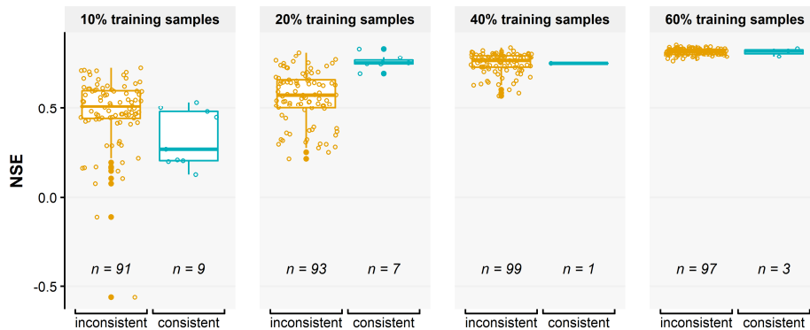
Figure 9 Boxplot of the prediction accuracy of the Washington Street SuDS site (WS) models when different sizes of samples are used in model training. For each sample size, the models that offer consistent and inconsistent explanations are grouped together, and the numbers of consistent and inconsistent models (the n values) are shown. Observational SHAP values were used in the computation. The points show the NSE of each model and their horizontal positions are randomly set to avoid overlapping.
