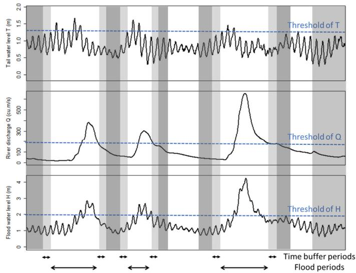
**Figure 5** Conceptual illustration of censored continuous simulation for simulating compound flood level H in estuarine regions caused by high tail water level in the ocean T and large river discharge Q. The time periods highlighted in dark grey are low water level periods; while the remaining time periods are high water level periods, which include flood periods and the time buffer.
