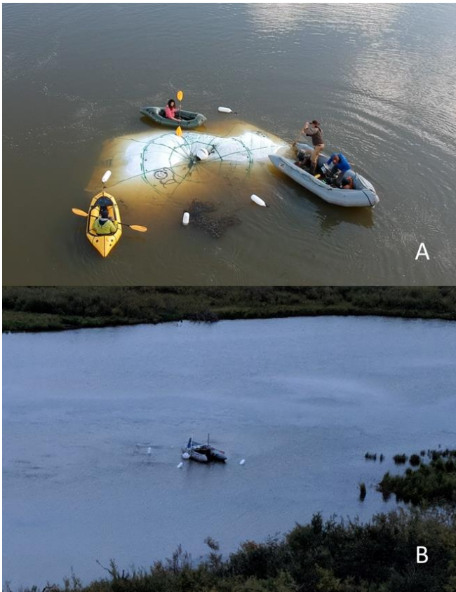
Figure 4: Bubble trap shown during installation before it was submerged (A) and during operation (B); the inflatable boat contained the measurement device at the center of the submerged bubble trap (Credit: O. Irzak).
