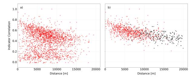
Figure 5. Indicator correlations for 1h temporal resolution and  $\alpha = 0.99$  between the secondary network and the nearest primary network stations before (left) and after (right) applying the filter (red Xes). The black dots refer to the indicator correlation between the primary network stations.
