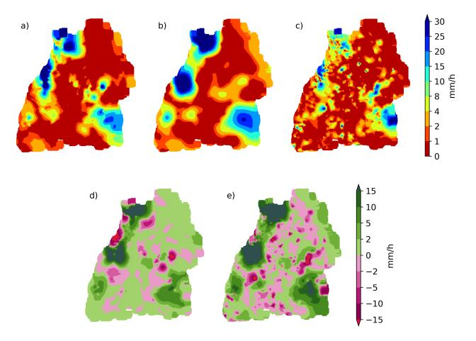
**Figure 6.** Interpolated precipitation for the time period 15:00 to 16:00 on June 11, 2018 (upper panel), and the differences between primary and combination, and primary and secondary data based interpolations. Panel a) shows the result after applying the filtering, b) the interpolation from the primary network and c) the one from the secondary network. Panels d) and e) depict the differences between b) and a) and b) and c) respectively.
