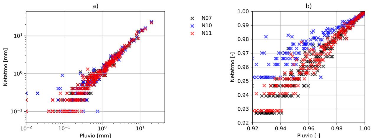
**Figure 3.** Scatter plot showing a) the hourly rainfall values (axes log-scaled) and b) the corresponding upper percentiles  $> 0.92$  (right) between the Pluvio<sup>2</sup> weighing gauge and three Netatmo gauges (N07, N10, N11) at the IWS Meteorological Station.
